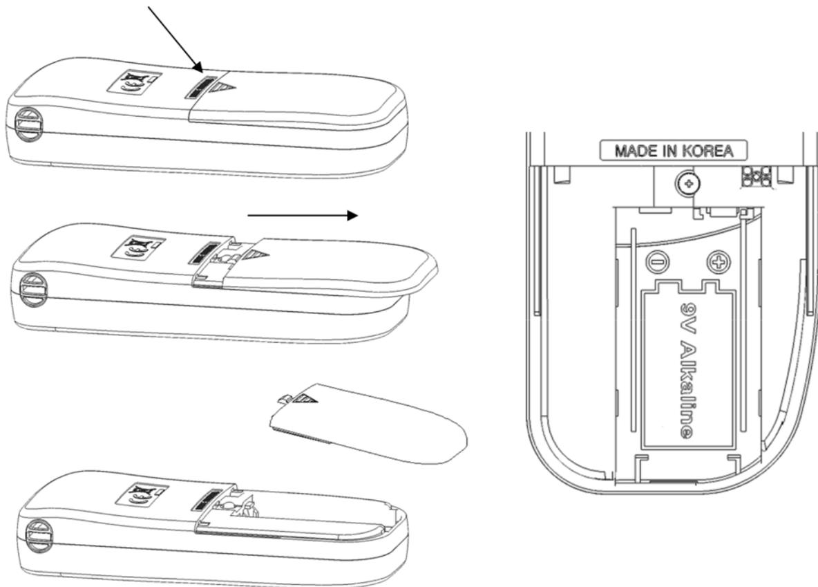
\*\*\* N.B. : Make sure to insert the battery with the proper position of positive(+) and negative(-) as indicated.
